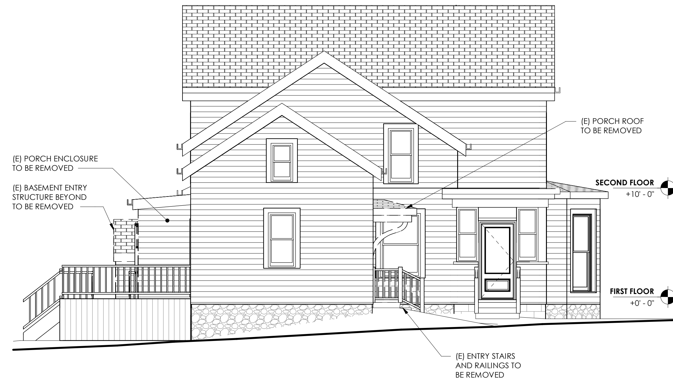
3 EXISTING - SOUTH SIDE ELEVATION 3/16" = 1'-0"
