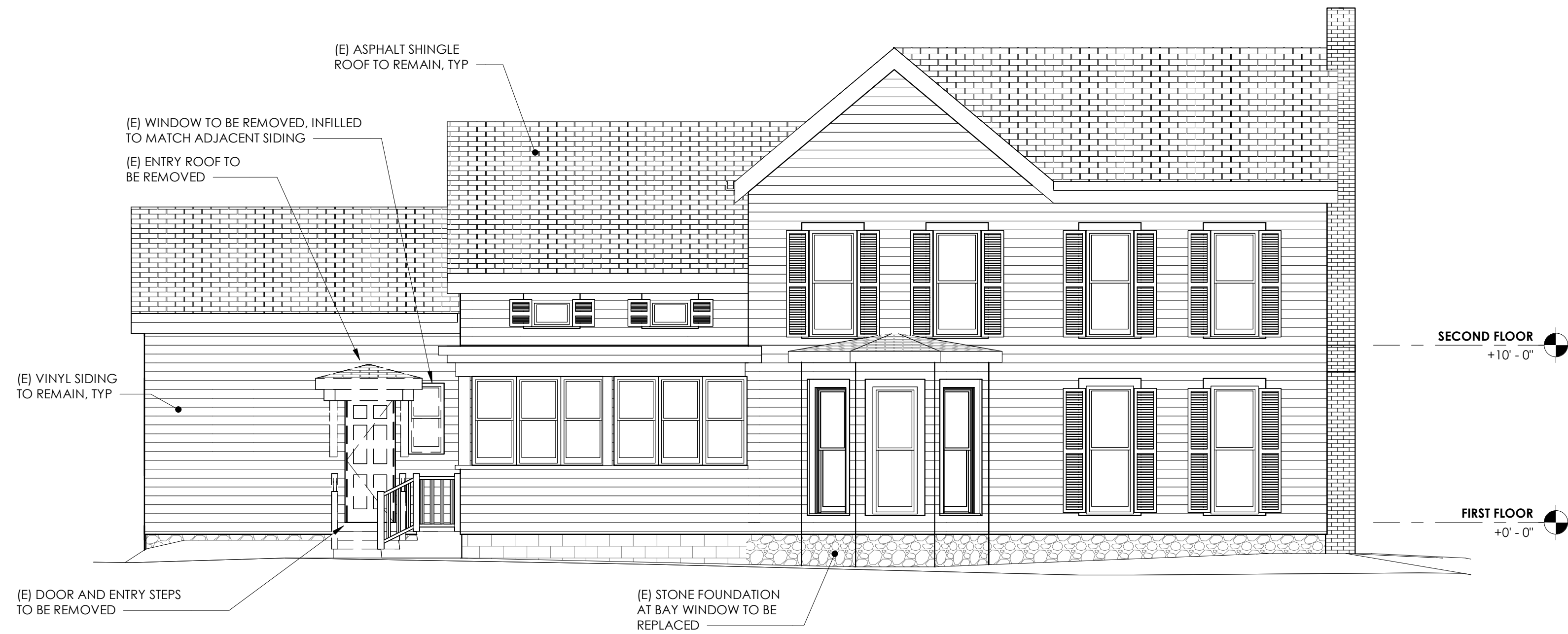
1 EXISTING - FRONT ELEVATION 3/16" = 1'-0"
