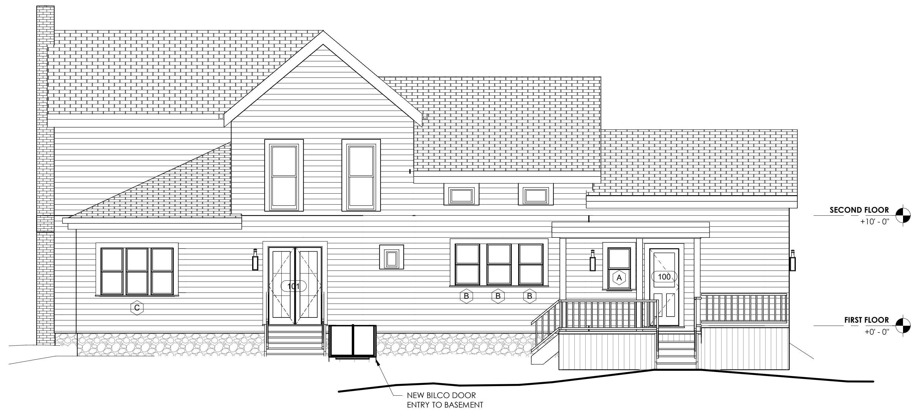
2 PROPOSED - REAR ELEVATION 3/16" = 1'-0"
