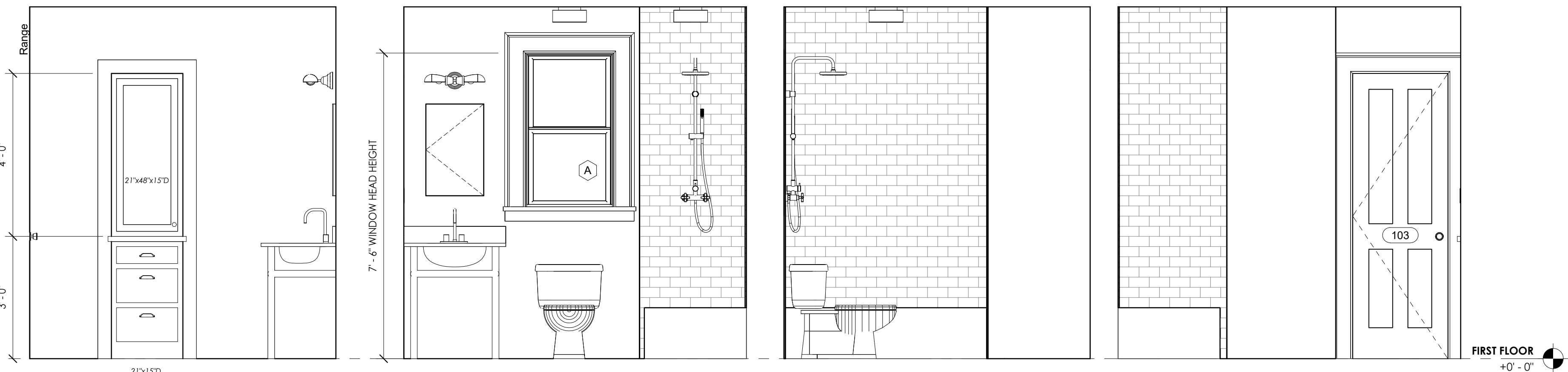
5 BATH 1 - ELEVATION A 1/2" = 1'-0"
