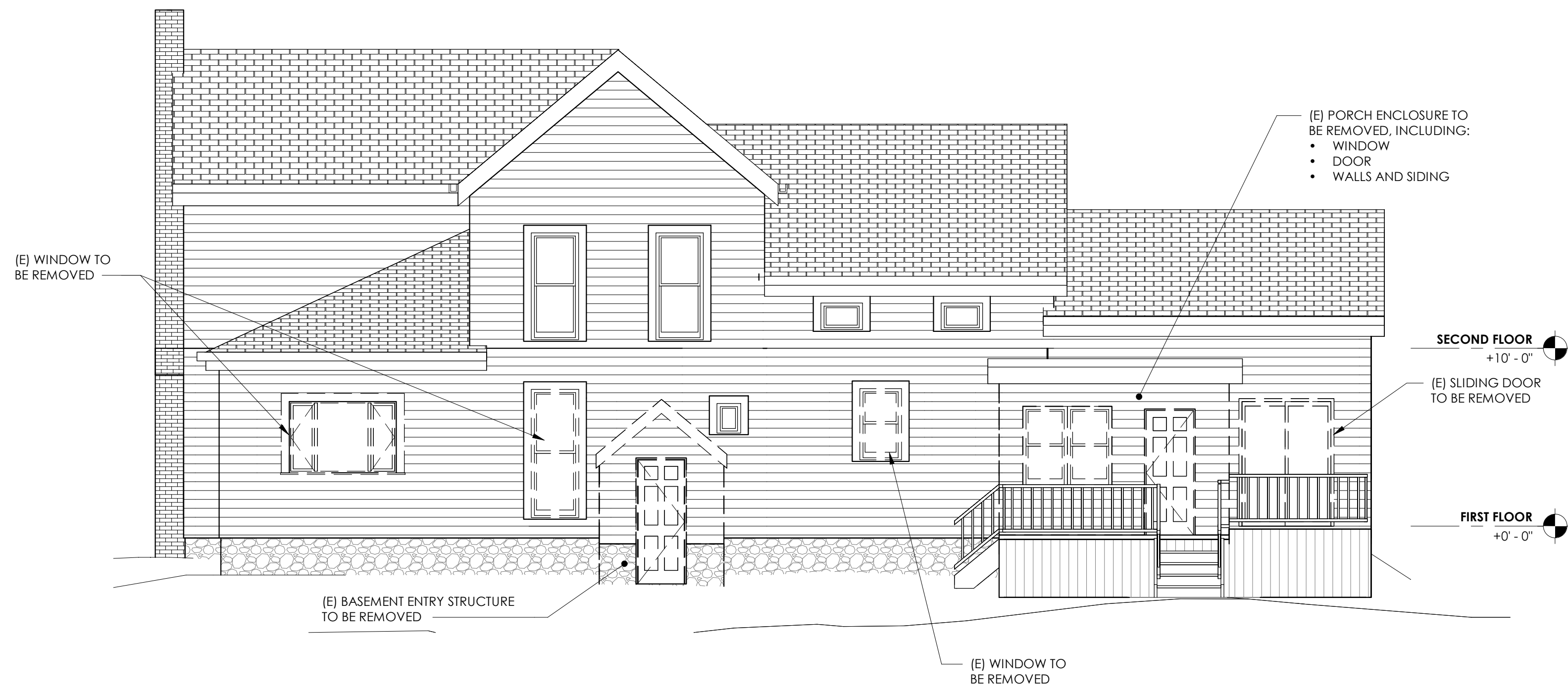
1 EXISTING - REAR ELEVATION 3/16" = 1'-0"
