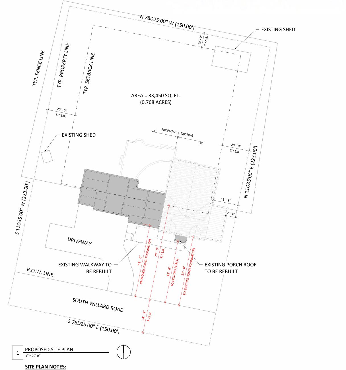
1. THIS PLAN IS TAKEN FROM AN INSTRUMENTAL SURVEY MAP COMPLETED BY TRIPLE POINT LAND SURVEYING, LLC. TITLED '78 WILLARD ROAD' (JOB NO. 0420-22) COMPLETED ON MAY 2, 2022. 2. ALL CONSTRUCTION TO BE LOCATED WITHIN BUILDABLE ENVELOPE WITH RESPECT TO ALL APPLICABLE SETBACKS INCLUDING, BUT NOT LIMITED TO, SIDE, FRONT & REARYARD SETBACKS. 3. ALL SEPTIC, DRIVEWAY, UTILITY, AUXILIARY STRUCTURES & CONSTRUCTION SHALL BE PER MUNICIPAL ZONING & ADOPTED BUILDING CODE AND/OR JURISDICTIONAL REGULATIONS AS
