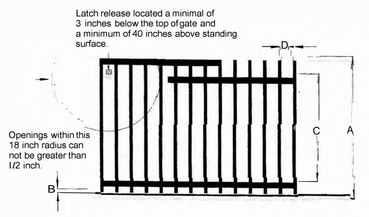
Dimension "A" must be 48 inches minimum from a standing surface to the top of gate. Dimension "B" may be 2 inches maximum from standing surface to the bottom of gate. If dimension "C" is less than 45 inches, dimension "D" cannot be greater than 1-3/4 inches. Dimension "Dn can never be greater than 4 inches.
