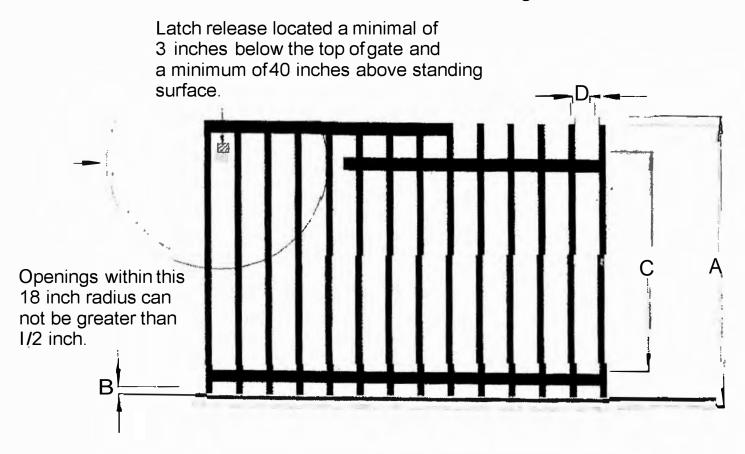
Dimension "A" must be 48 inches minimum from a standing surface to the top of gate. Dimension "B" may be 2 inches maximum from standing surface to the bottom of gate. If dimension "C" is less than 45 inches, dimension "D" cannot be greater than 1-3/4 inches. Dimension "Dn can never be greater than 4 inches.
