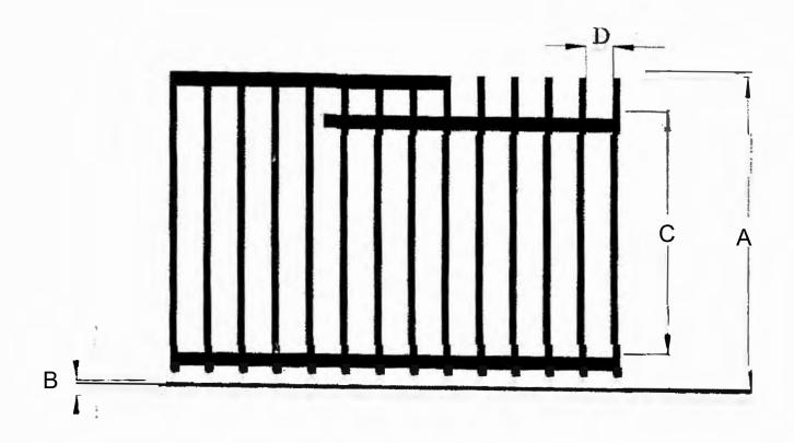
Dimension "A" must be 48 inches minimum from a standing surface to the top of gate. Dimension "B" may be 2 inches maximum from standing surface to the bottom of gate. If dimension "C" is less than 45 inches, dimension "D" cannot be greater than 1-3/4 inches. Dimension "D" can never be greater than 4 inches.
