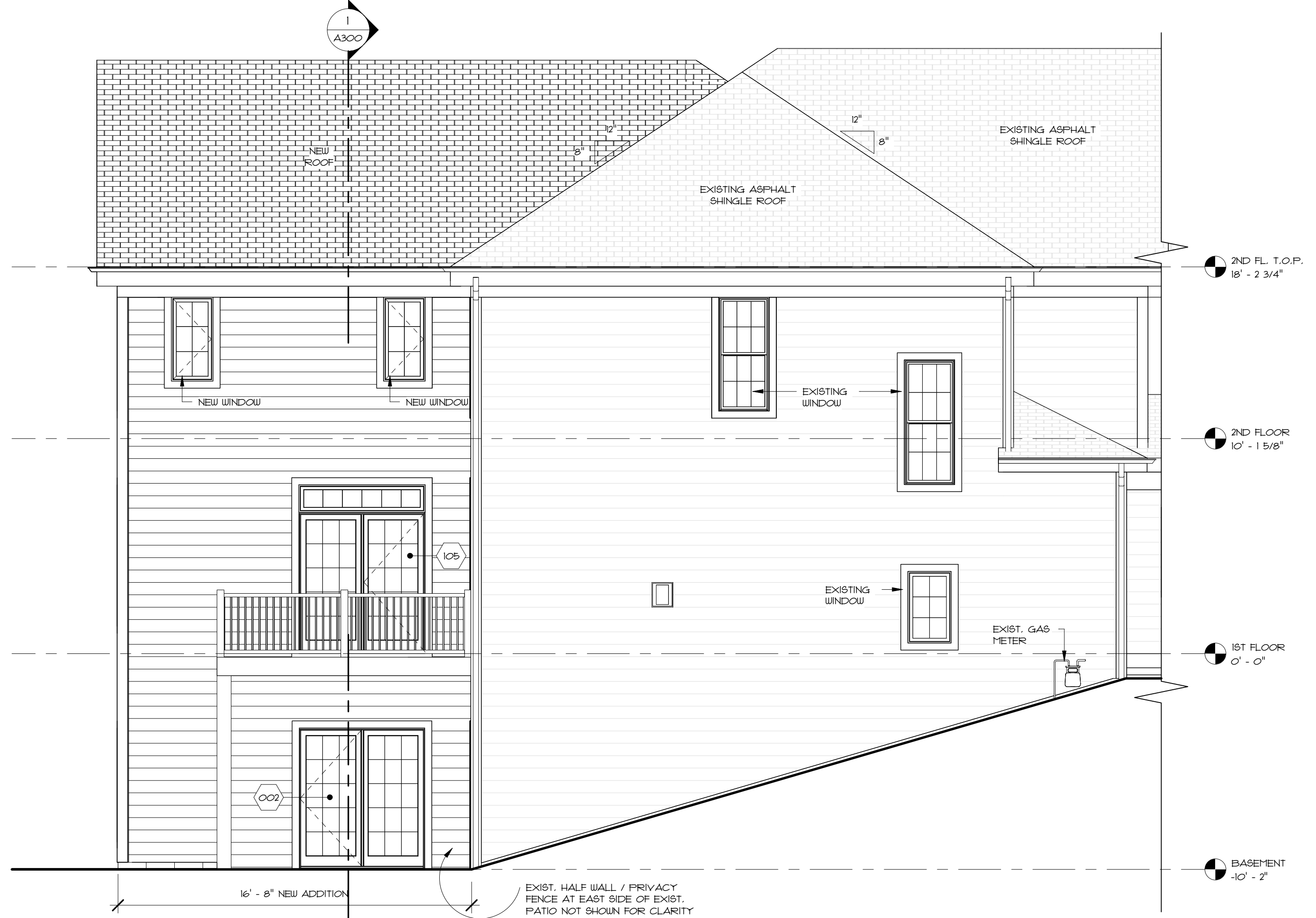
3 EAST ELEVATION SCALE: 1/4" = 1'-0"
