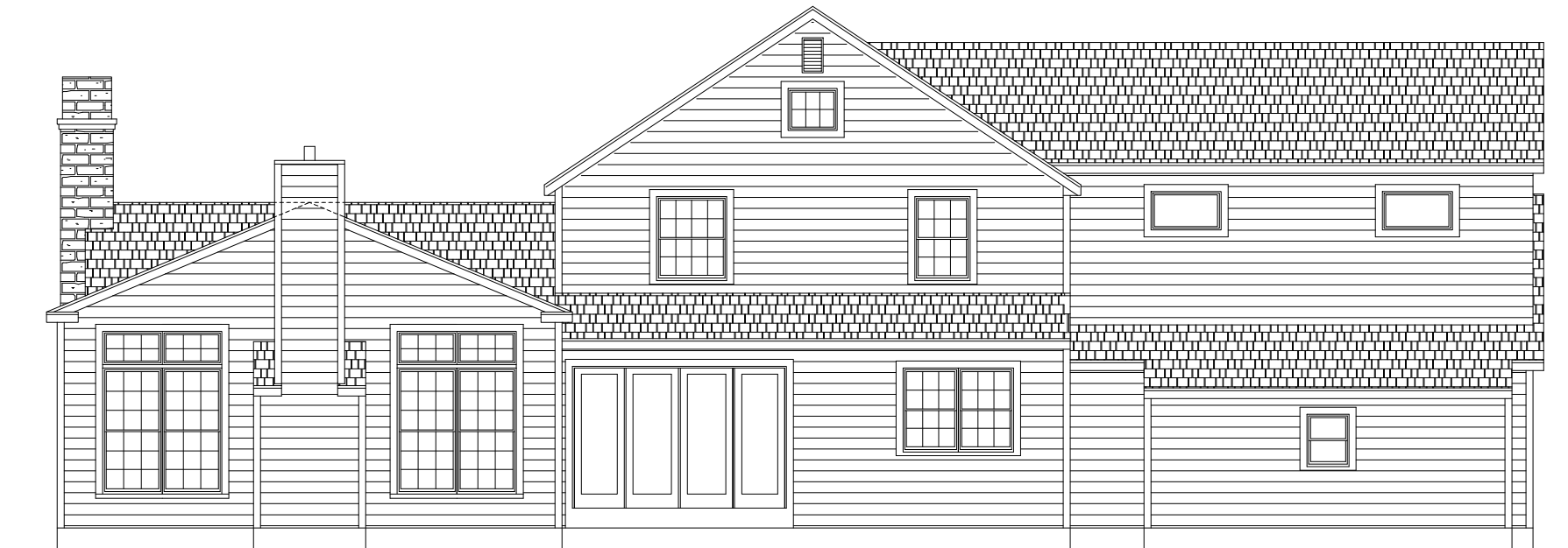
EXISTING REAR ELEVATION
