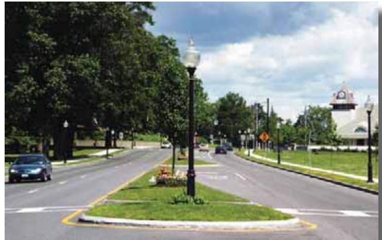
Planted median slows traffic on this state highway and creates an attractive gateway to downtown Saratoga Springs.
