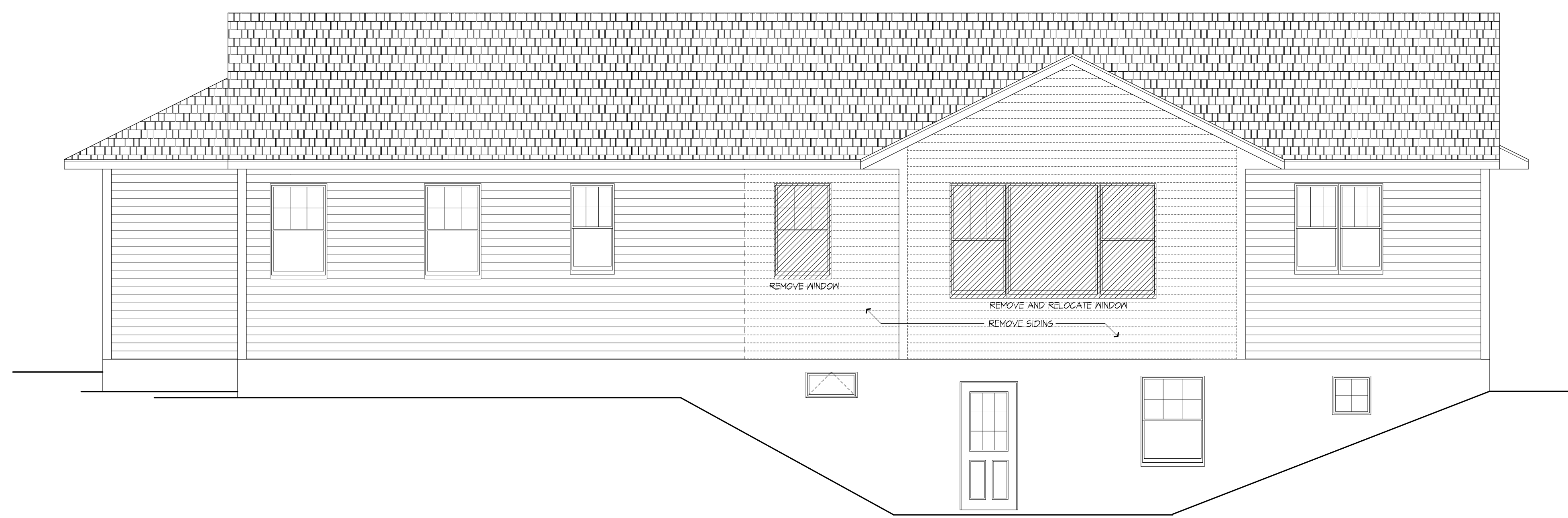
REAR ELEVATION EXISTING WITH REMOVALS SHOWN
