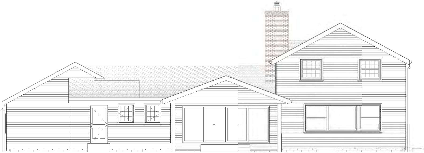
1 BACK ELEVATION NEW - DESIGN REVIEW (P3) 1/8" = 1'-0"
