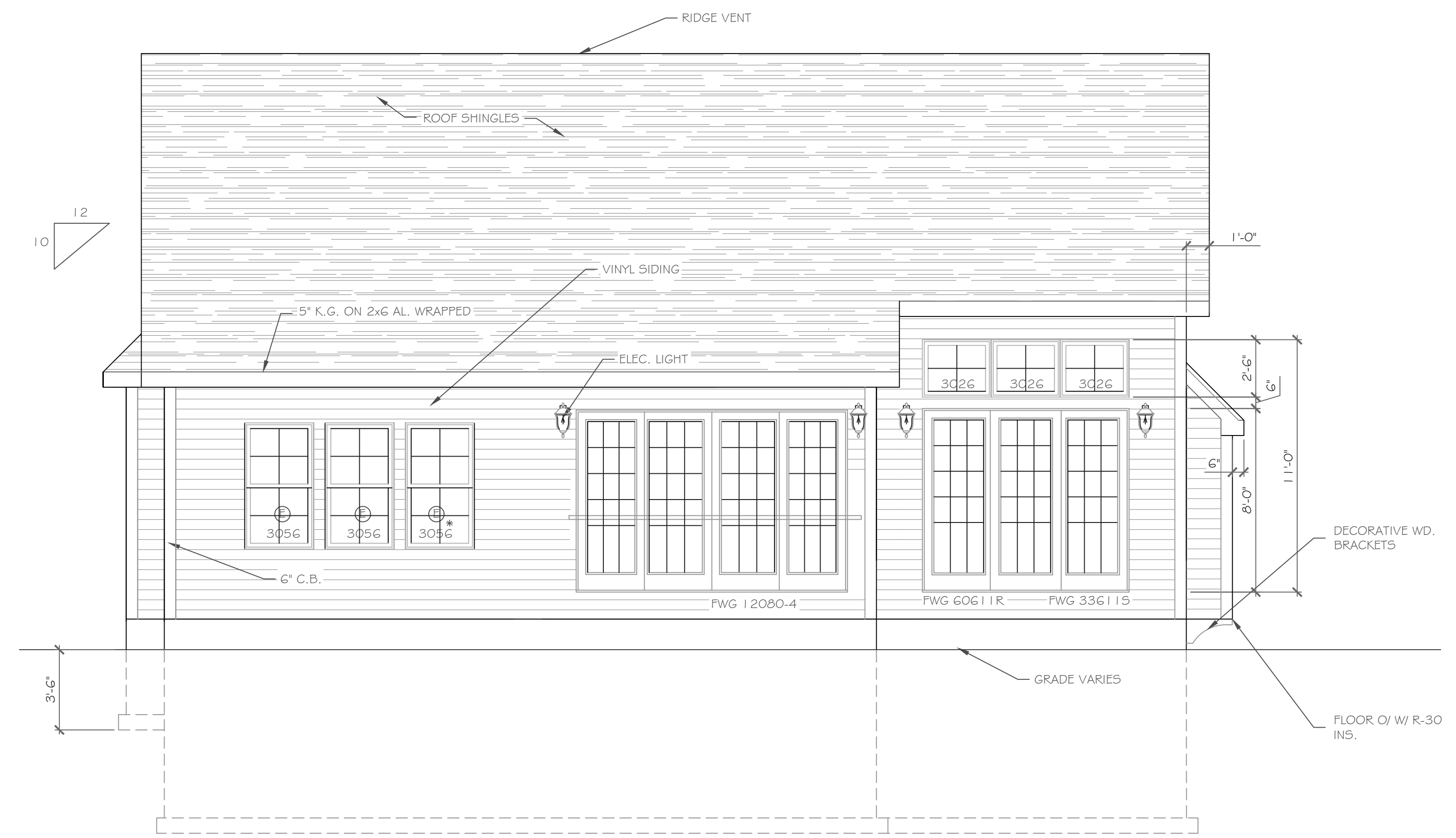
REAR ELEVATION SCALE: 1/4" = 1'-0"
