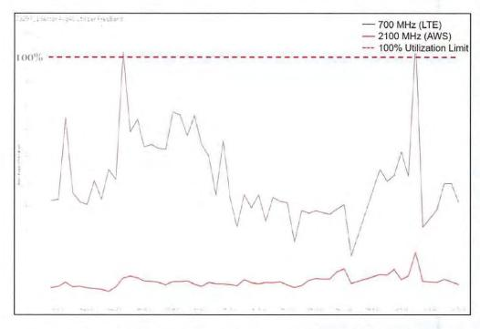
**Summary**: This graph shows AvgAC (Average Active Connections). AvgAC utilization by carrier is a measurement of max active connection capacity per sector in any given time slot. When this limit is reached, no additional devices will be able to connect to the site, resulting in connection failures and dropped calls.
