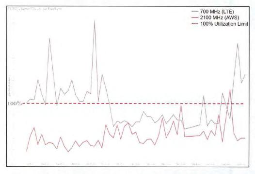
**Summary**: This graph shows FDV (**F**orward **D**ata **V**olume) which is a measurement of the customer data usage that this sector currently serves. As this limit is approached, data rates slow to unacceptable levels, potentially causing unreliable service for Verizon Wireless customers.
