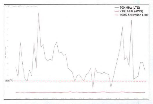
**Summary**: This graph shows ASEU (**A**verage **S**chedule **E**ligible **U**ser). ASEU is a measurement of the loading of the control channels and systems of a given site. The ASEU load is heavily impacted by distant users or those in poor RF conditions.
