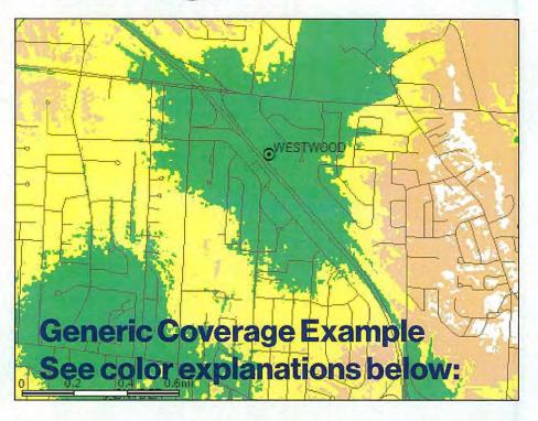
**Coverage** is best shown via coverage maps. RF engineers use computer simulation tools that take into account terrain, vegetation, building types, and site specifics to model the RF environment. This model is used to simulate the real world network and assist engineers to evaluate the impact of a proposed site (along with industry experience and other tools).
