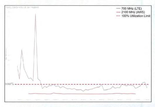
**Summary**: This graph shows ASEU (**A**verage **S**chedule **E**ligible **U**ser). ASEU is a measurement of the loading of the control channels and systems of a given site. The ASEU load is heavily impacted by distant users or those in poor RF conditions.
