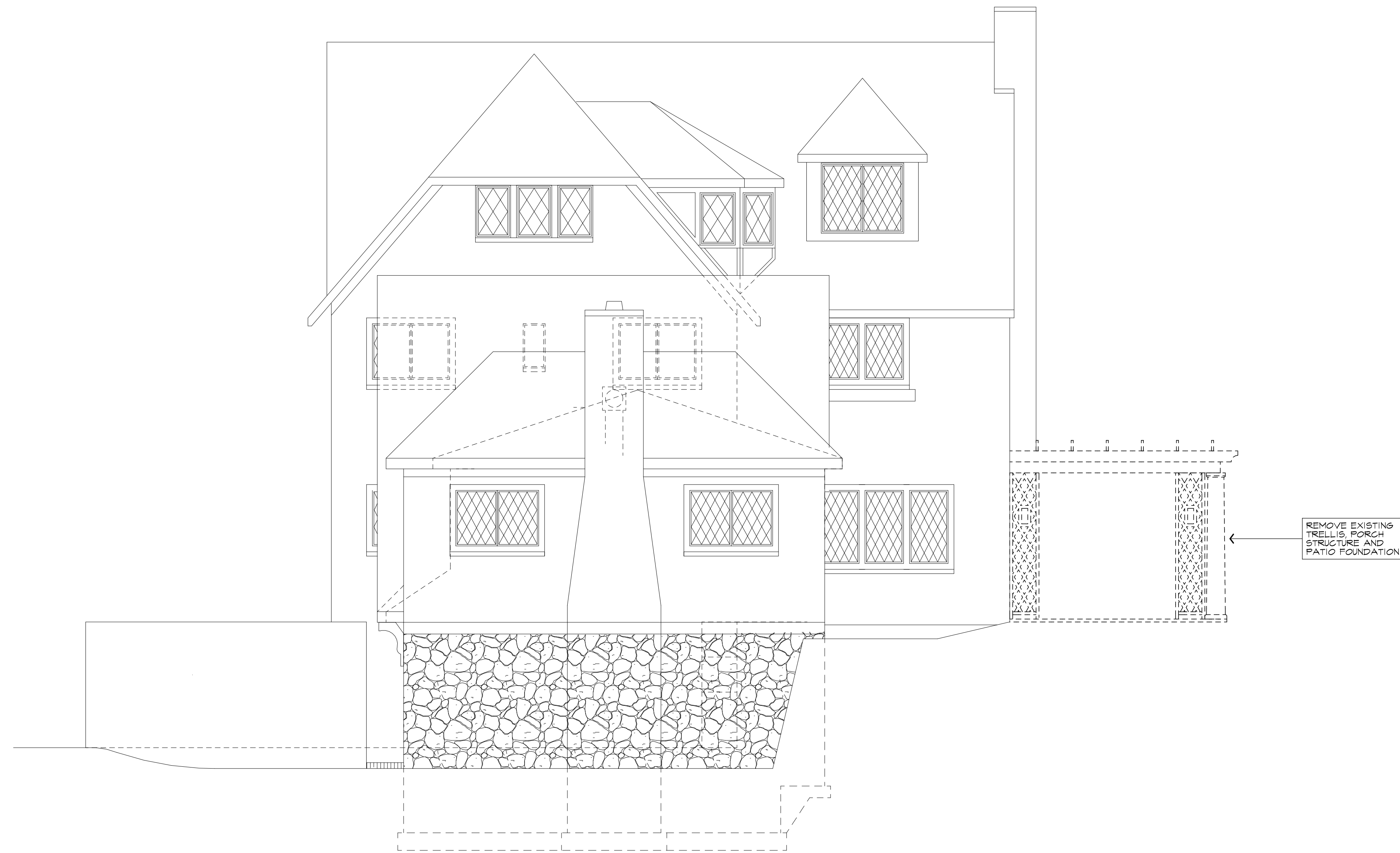
REAR ELEVATION/ EXISTING WITH REMOVALS SHOWN
