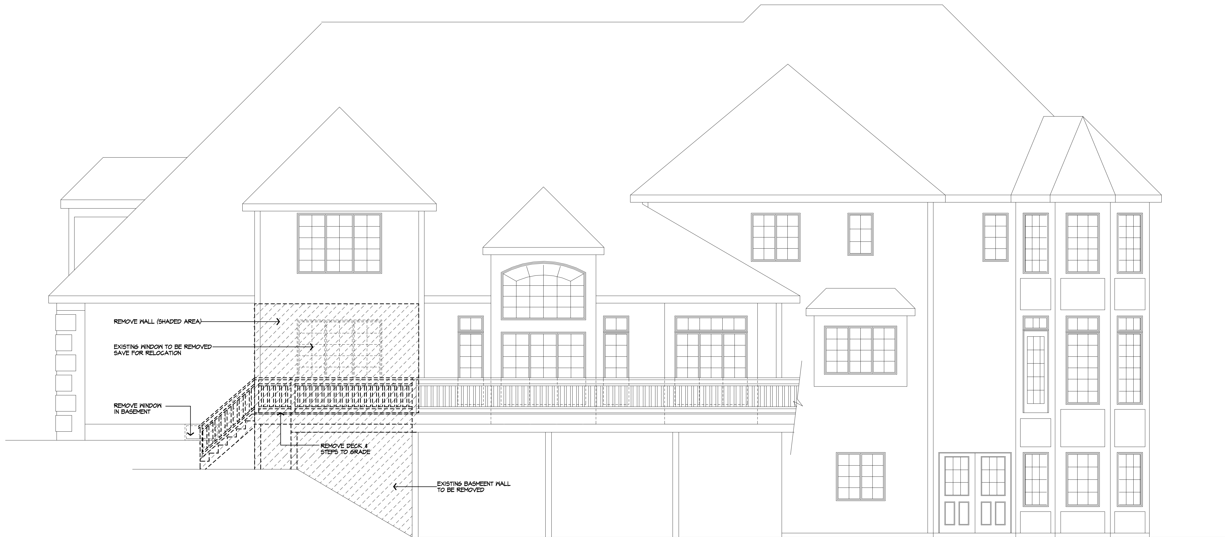
REAR ELEVATION / EXISTING WITH REMOVALS SHOWN
