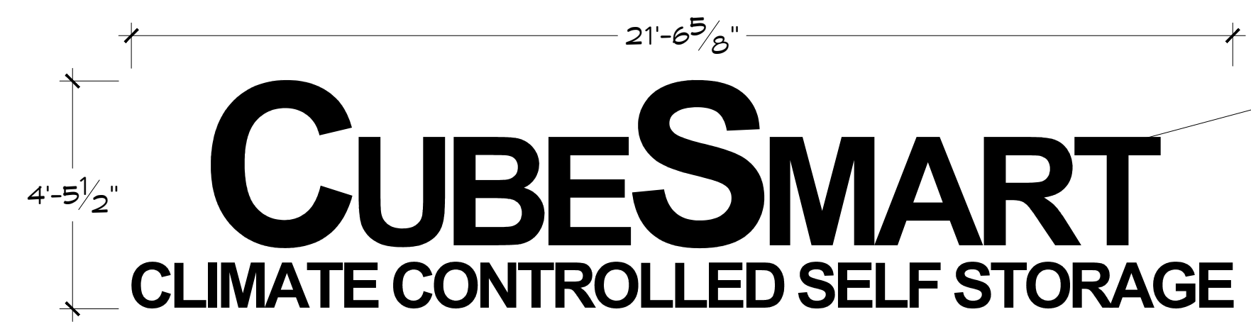
5 RACEWAY MOUNTED INTERNALLY LIT SIGN SCALE: 3/8" = 1' - 0"
